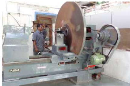
Lathe Machine upto 2.5 m plate OD
