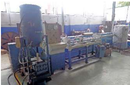
Hydrotest Rig upto 6" line size and pressure upto 80kg/cm 2
